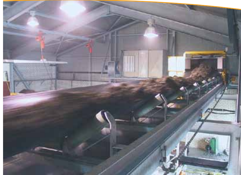
High speed loading of tunnel filling machines and cassettes for phase II and III tunnels as well as truck loading.
